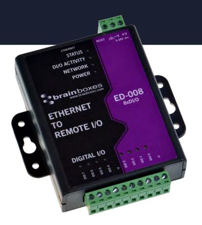
Connect digital sensors & transducers to bring data onto the network
